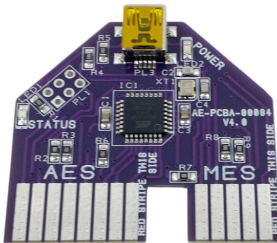
The Display Tester is designed to check that your Series 8000 display and ribbon cable are working correctly. It will help you establish whether your display is faulty or not, or whether the issue lies elsewhere with your fridge. Please note that the Display Tester does not have any function to operate the fridge.
