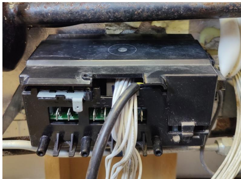
Unplug the 20 way connector and plug connector #1 of the replacement loom in place of the old one.
