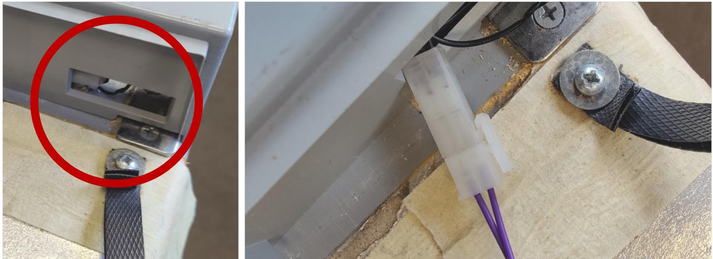
**Step 6:** Remove the front plastic fascia (control PCB housing) from the fridge to access and unplug the existing 8 way connector. Feed connector #5 through the same access hole as is **Step 5**.
