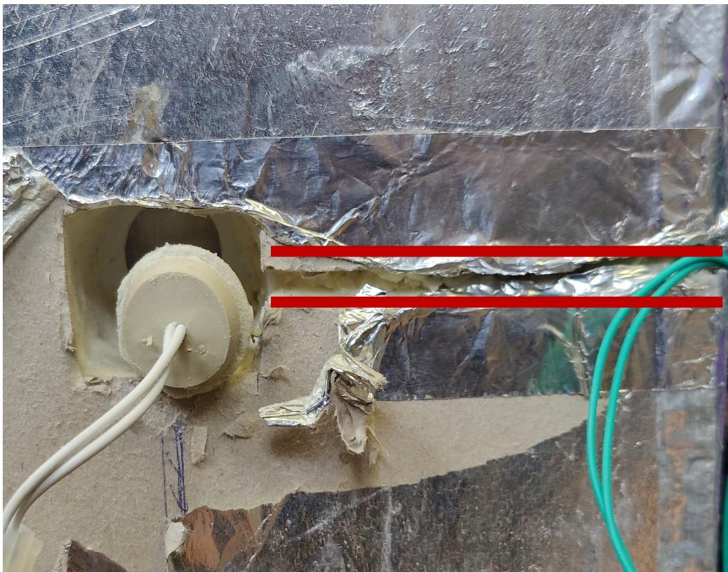
Feed connector #2 through the hole of the removed seal, plug the connector end in to the internal mating half and tuck fully into the carved channel. Refit the seal and cover the cut-out with foil tape.
