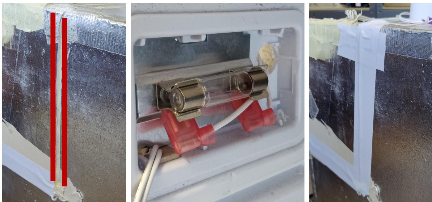
**Step 5:** Inside the plastic housing that holds the fascia at the top front of the fridge, is the door sensor connector. Through the access hole, unplug the existing connector and attach connector #3 in its place.
