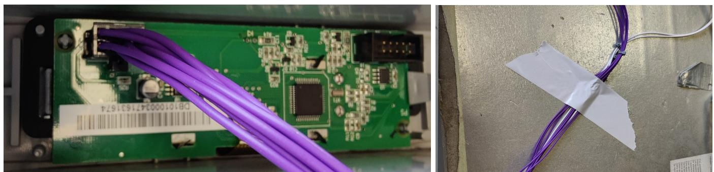
**Step 7:** Once all previous steps have been followed, ensure that no wires hang over, or stick out the side, and check that all the wires have been secured. Before refitting the fridge, power on, and test it. Once tested, it can be refitted - ensure the replacement loom is tucked in at the sides to avoid damage
