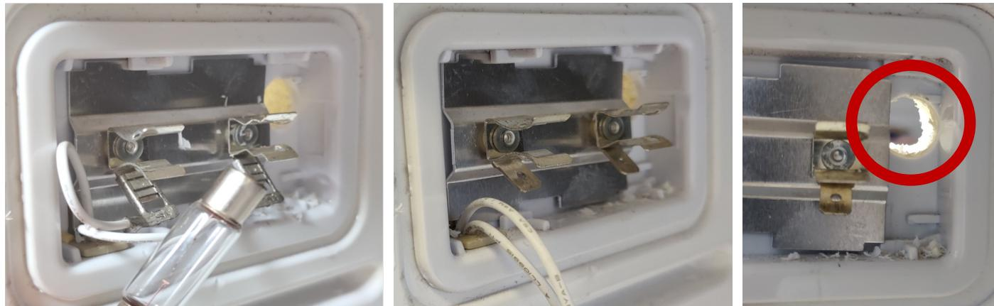
Carve a channel vertically from the top of the fridge down to the hole. Attach connectors #4 (Flag x2) to the bulb holder - it does not matter which blade connects to which terminal. Gently pull the wires taut through the hole from the exterior and run them up the channel. Cover up with foil tape ensuring the side of the fridge is flat and flush.
