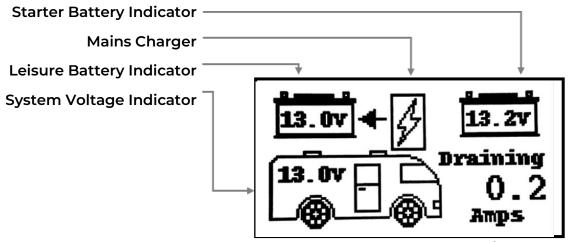
STARTER BATTERY INDICATOR shows Starter Battery VOLTAGE, if connected.
