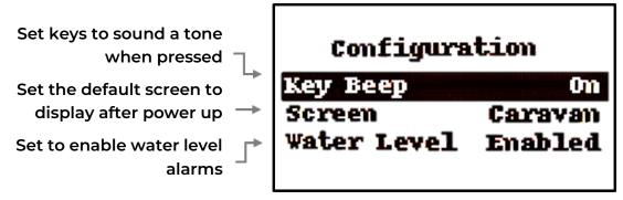
If the vehicle does NOT have tank sensors, water level alarms should be DISABLED.
