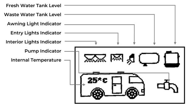
FRESH & WASTE WATER TANK LEVEL displays fill level in quarter increments. Tank level on screen will indicate tank fill level by how much of the indicator is filled in.
