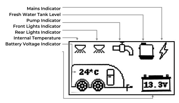
MAINS INDICATOR signals that MAINS has been detected.
