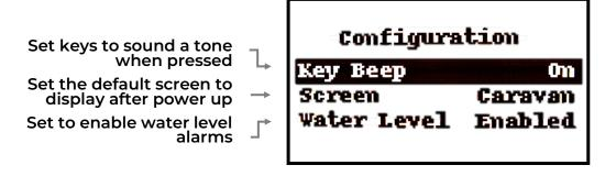
If the vehicle does NOT have tank sensors, water level alarms should be DISABLED.
