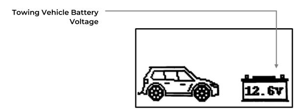
TOWING VEHICLE SCREEN is only available when a towing vehicle is connected.
