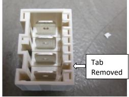
4. Locking latch - On the wiring loom connector there will be a locking latch down the centre of the connector. If this does not fit in between other connectors, when fully inserted into the PCB, then the latch will need to be cut off. If there is no restriction, the latch can remain as shown below.
