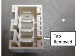
2. Locking latch - On the wiring loom connector there will be a locking latch down the centre of the connector. If this does not fit in between other connectors, when fully inserted into the PCB, then the latch will need to be cut off. If there is no restriction, the latch can remain as shown below.
