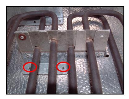
Drill out the two pop rivets in the metal L bracket holding it to the back (DO NOT remove the silvery mica spacers at this stage). You may find that the mica spacers are very badly damaged, in which case
