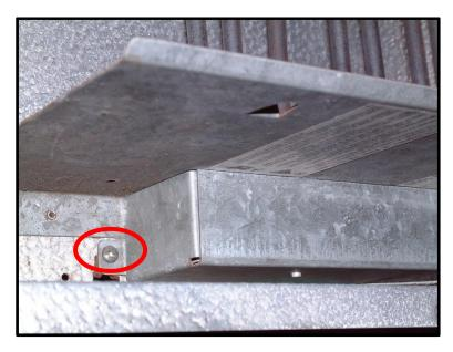
You can now see the elements as shown above. Remove the single screw at the bottom of the cover and slide the cover up and across to remove it.
