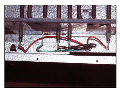
Pull off the 4 electrical connections from the ends of the elements noting the position each is connected to. There is no need to remove the green earth connection.
