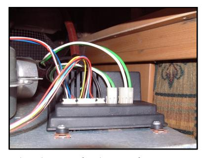
Remove the five 12V electrical connections from the main unit for ease or removing parts and to avoid damage. These are easily replaced later as they are polarised so you cannot fit the wrong one in the wrong location. You also need to remove the 'Kettle style' mains input cable from the bottom of the unit.
