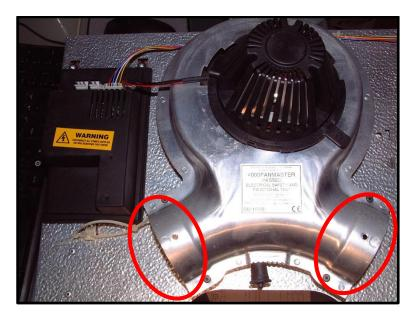
Remove the two outlet ducts from the motor housing, as shown above, by removing the two screws and pulling out.
