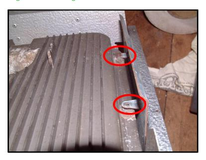
Remove the 5 bolts holding the large cast gas heat exchanger (the elements are behind) and remove the heat exchanger complete with thermostats/bulb, shaft and control knob.
