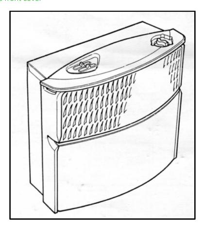
Remove front cover (be very careful as the slider control is still attached – disconnect carefully). This is achieved by pulling the bottom of the fire front away from the back and then lifting the top of the cover off the controls.
