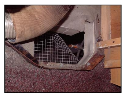
Isolate the gas supply. From underneath the vehicle remove the gas pipe by undoing the nut on the elbow fitting and pulling the pipe out from the elbow. The picture above shows the position of the gas pipe with the heater removed for clarity.
