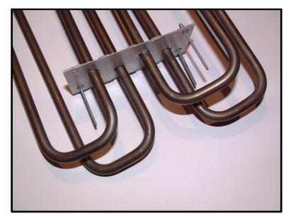
Position the new elements (either way round – they are identical) into the mica supports and temporarily hold with bulldog clips or similar if required. Assemble the Mica supports and elements with the metal mounting bracket as shown. Using 3x6mm pop rivets reattach the Mica supports and metal bracket not forgetting the washer on the upper pop rivet. Refit the clip to the Mica support if fitted.
