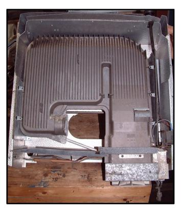
All the external connections and wiring should now be removed from the unit. **WARNING – heavy**. This should allow complete removal of the unit from the vehicle. Remove the unit and initially lay front down on a suitable workbench (picture shows unit the front up).
