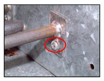
Remove the 4 screws attaching the element ends to the bulkhead
