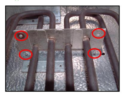
Drill out the rivets/remove the clip from the two mica spacers to separate/free the two elements (USE EXTEME CAUTION as the mica is brittle!). Retain the clips and/or washer from the Mica for use in reassembly
