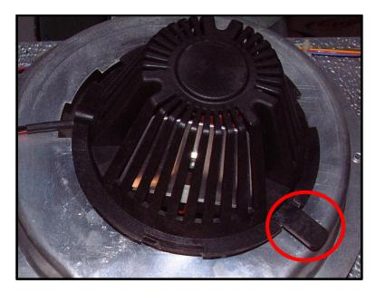
You need to work on the unit with the front upwards. However the back of the unit it not very flat. In order to avoid damage and provide a stable heater, first remove the fan unit by lifting the black tab, rotating the unit anti-clockwise and then withdrawing the motor and fan as a complete unit. Now is a good time to clean/vacuum the fan, motor and fan chamber to remove dust/dirt.
