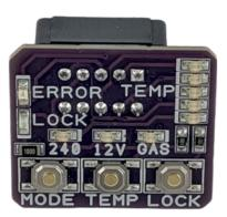
This test display is intended to provide the same functionality as the original display, but plugs directly onto the main PCB at the back of the fridge. This allows control of the fridge whilst probing/testing, avoiding the need to go back to the front of the fridge to change modes/settings.
