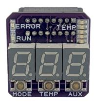
The test display is intended to provide the same functionality as the original display, but plugs directly onto the main PCB at the back of the fridge. This allows control of the fridge whilst probing/testing, avoiding the need to go back to the front of the fridge to change modes/settings.
