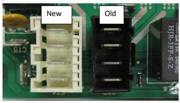
Many PCB's were fitted with RAST5 connectors made by Molex. Molex has now made these connectors obsolete so manufacturers have had to use an alternative RAST5 connector which differs from the original. The photo above shows the old and new connectors positioned the same way round as each other. The new connectors give 2 issues depending on the PCB manufacturer and loom connectors.
