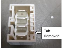
2. Locking latch - On the wiring loom connector there will be a locking latch down the centre of the connector. If this does not fit in between other connectors, when fully inserted into the PCB, then the latch will need to be cut off. If there is no restriction, the latch can remain as shown below.
