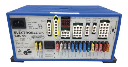
To fit the test plug, remove the existing loom connector by squeezing the tabs on the side of it. In place of the connector removed, fit the test plug onto the EBL. Now plug the loom connector into the back of the test plug.
